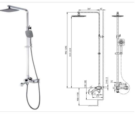
56 3700C Wall-Mounted Mixer with Diverter 35 mm Ceramic Cartridge ø22x88mm, Turned Diverter, 180° Three Ways G1/2" Outlets and Inlets Chrome Finish
