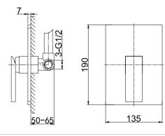
35 4700-1C Wall-Mounted Mixer without Diverter 35 mm Ceramic Cartridge One Way G1/2" Outlets and Inlets Chrome Finish
