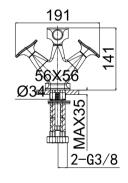
65 3103C **Double-Handle Bath Mixer** G1/2"x38.5 Ceramic Cartridge M32x8 Hidden Aerator M20x1 Automatic Diverter G1/2"S-Shaped Connections 3/8" Connecting Hoses **Chrome Finish**
