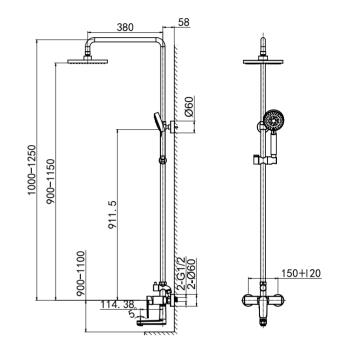
26 3602C Shower/Bath Combination 35 mm Ceramic Cartridge M18.5x1 Female Thread Aerator ø28x72 mm, Turned Diverter, 360° G1/2" S-Shaped Connections Chrome Finish
