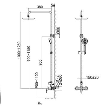
28 4700C Wall-Mounted Mixer without Diverter 35 mm Ceramic Cartridge Chrome Finish
