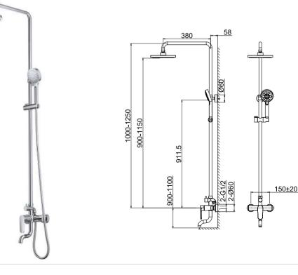
26 3700C Wall-Mounted Mixer with Diverter 35 mm Ceramic Cartridge ø22x88 mm, Turned Diverter, 180° Two Ways G1/2" Outlets and Inlets Chrome Finish
