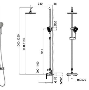
26 4700C Wall-Mounted Mixer without Diverter 35 mm Ceramic Cartridge One Way G1/2" Inlets Chrome Finish
