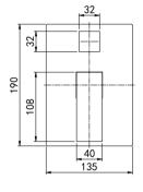
35 3700-1C Wall-Mounted Mixer with Diverter 35 mm Ceramic Cartridge ø22x66 mm, Turned Diverter, 180° Two Ways G1/2" Outlets and Inlets Chrome Finish
