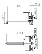
26 3601C Shower/Bath Combination 35 mm Ceramic Cartridge M24x1 Male Thread Aerator ø28x72 mm, Turned Diverter, 360° G1/2" S-Shaped Connections Chrome Finish
