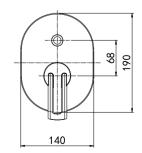
32 3601C Shower/Bath Combination 40 mm Ceramic Cartridge M28x1 Male Thread Larmina Swiveled Spout ø33x57.5 mm, Turned Diverter, 360° S-Shaped Connections Chrome Finish
