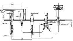
56 3601C Shower Combination 35 mm Ceramic Cartridge M24x1 Hidden Aerator Swiveled Spout ø22x46 mm, Turned Diverter, 180° M22x1.5x49 mm Diverter G1/2" S-Shaped Connections Chrome Finish
