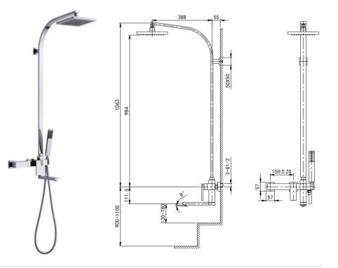
35 3602C Shower/Bath Combination 35 mm Ceramic Cartridge M24x1 Male Thread Aerator Swiveled Spout ø34.5x54 mm, Turned Diverter, 360° G1/2" S-Shaped Connections Chrome Finish
